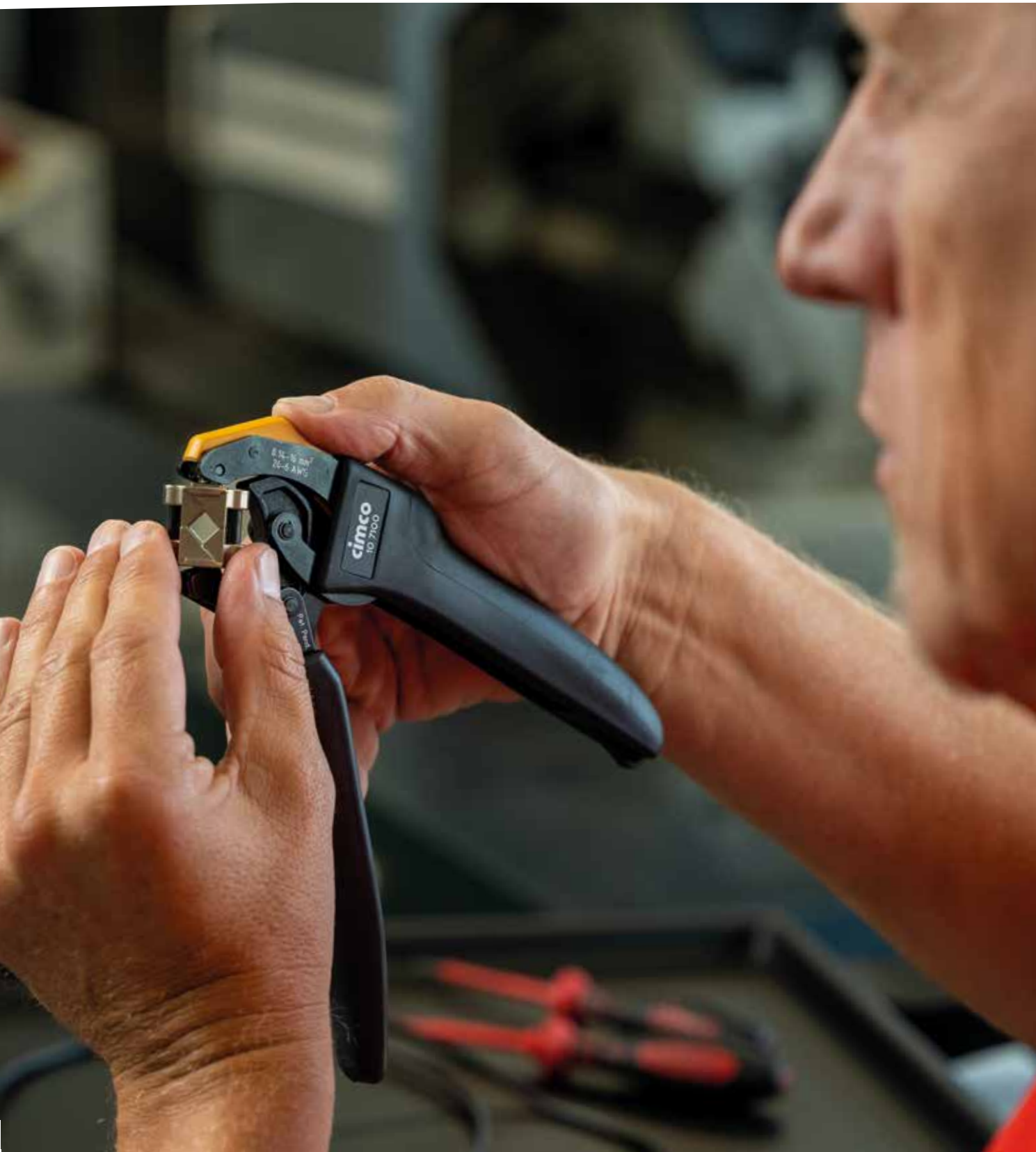
Flexible to use: thanks to a die that rotates without needing tools, the POWER-CRIMP TWIST is the ideal tool for working in confined installation spaces.
