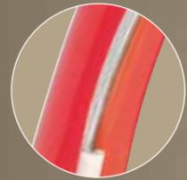
Handle sleeves with two-coloured plastic dip insulation (if the red layer is damaged and the orange layer is visible, the insulation is no longer providing a protective function).
