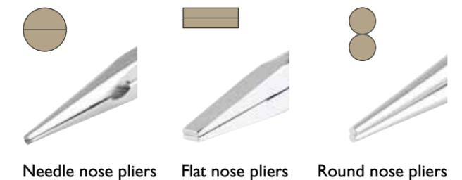
Needle nose pliers   Flat nose pliers   Round nose pliers
